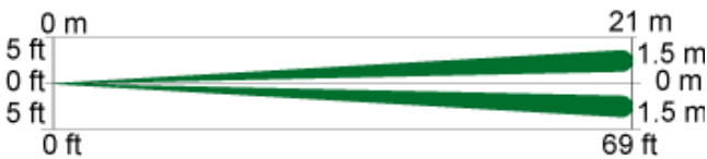
Top View Optional Long Range Coverage 21 m x 3 m Requires OMLR93-3 Long Range Mirror. Walking speed range is 0.2 m/s to 4.0 m/s.
